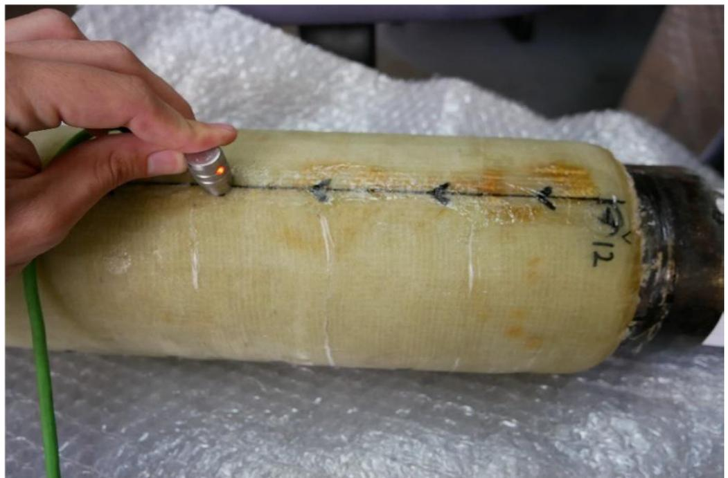
There are two distinct signatures relating to two types of flaws. The first was a delamination in the wrap layers, indicated by Gate 1 on the Bondascope shown at left. The second was a disbond between the composite structure itself and the steel pipe, indicated by Gate 2 shown at left. We delivered our findings to the pipe operator and they will be able to use this information to cut down on unnecessary repairs and focus only on areas that need attention.
