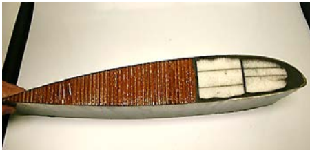
Carbon fiber skins with honeycomb core
