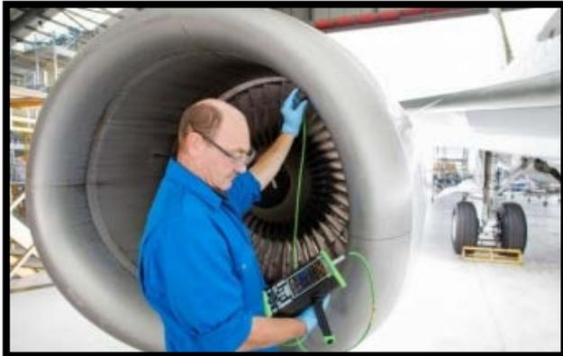
**Pitch-Catch | RF:** Transmits a short burst of acoustic energy into the part and measures the amplitude and phase change of the received signal. A disbond reduces material integrity and thus sound attenuation within the part leading to a higher amplitude at the receiver tip of the probe.
