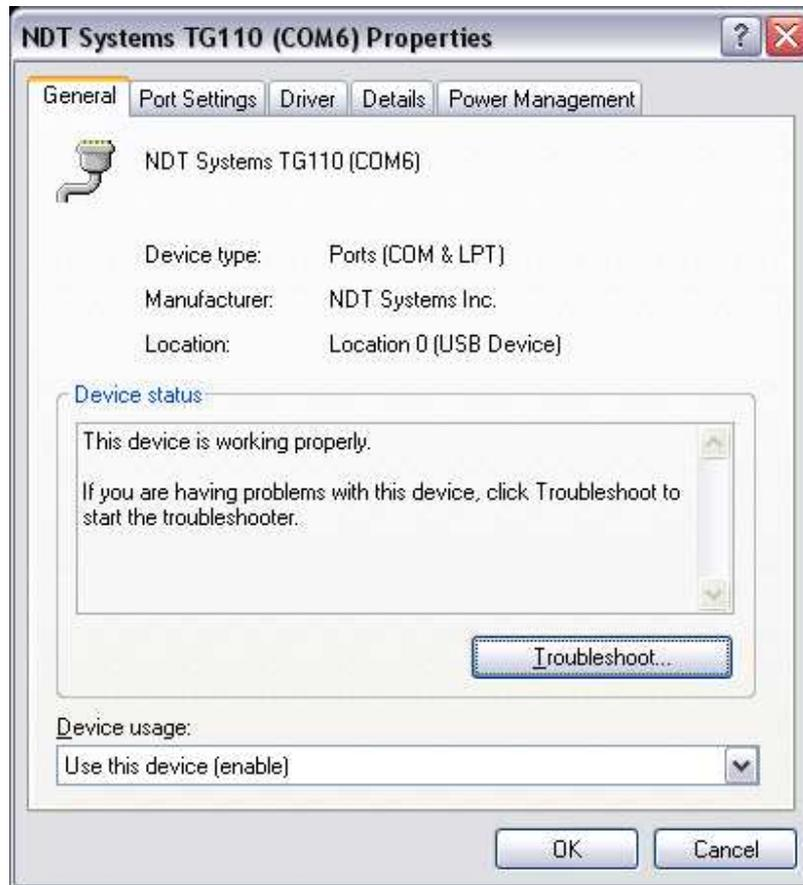
Click on the NDT Systems instrument listing to bring up its properties. If it is necessary to change the COM Port it is assigned to, click on the Port Settings tab.
