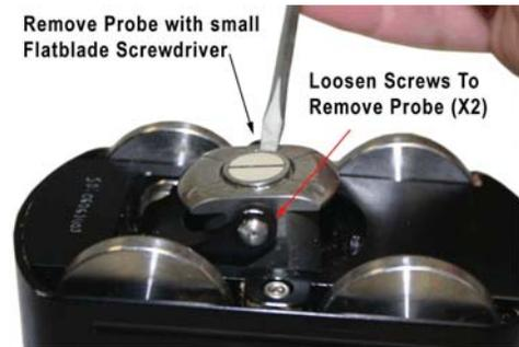
**Calibration:** Note - Quick Reference for the Ultrasonic Calibration is shown on back side of unit.
