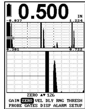
**However, note that T-readout did not change unless the gain was substantially increased. With TG400's digital electronics, it is not necessary to use the graticule or other precise settings of range in order to calibrate for, and to readout precise thicknesses.**
