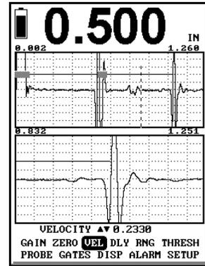
For precision thickness gaging, the type of waveform used for setups has a significant effect on gaging results. Note that the RECT default is +HW, meaning that the current display is of signals that are positive half-wave rectified.
