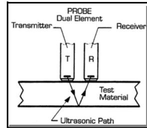
A dual element transducer is always in a "listening" mode as one half is transmitting. The real benefit with a dual can be found when inspecting corroded, pitted or eroded materials. Dual element transducer have the ability to discriminate the peaks and valleys of corrosion and or pitting.
