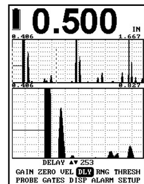
14. With the RANGE at 1.00 inch cursor to Select GATES from the MAIN Menu and select IP-BLK. The Up & Down arrow keys control the length of the blocking gate, referred to as "IP-BLK gate", and represented by the Thick dotted bar extending horizontally along the thickness gate line on the A-trace from the left-hand side of the
