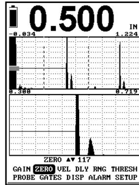
In our example, using a 0.500 inch thickness step, we have yet to perform any operations to "calibrate" the Thickness readout. Most probably the reading is close to 0.500 inch, since the FACTORY setup defaults are deliberately designed to produce nearly correct calibration for a contact transducer being used on steel having longitudinal sound velocity of 0.2330 inches/microsecond.
