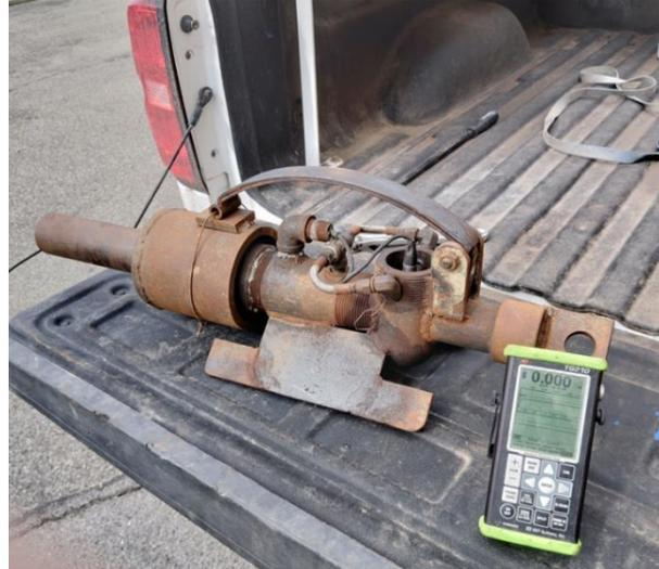
The TG-410 is set up for immersion testing by gating out the water path, and measuring the sound wave travel time from the water-pipe interface echo to the pipe backwall echo. Nominal thickness values for the pipe wall are close to 0.5", and displayed thicknesses significantly less are marked as potential flaws. For depths of 60' the TG-410 works very well, and the signal to noise ratio from interface to backwall is well defined.
